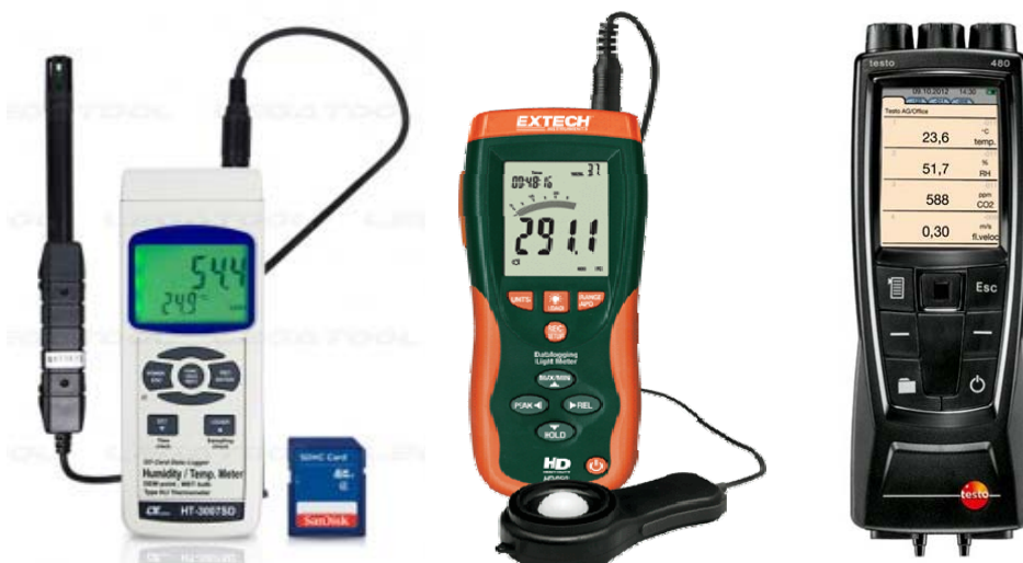
Figure 1: Measuring instruments (HT 3007SD – temperature and relative air humidity, Testo 480 - airflow velocity and HD450 - illumination)
