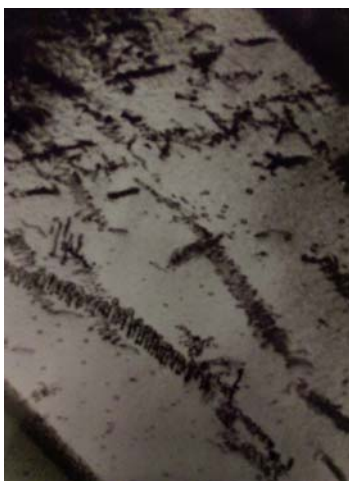
Figure 1. Microstructure of alloys in isothermal aging on the 175°C, zoom 24000X
