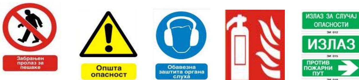
Picture 2: Examples of prohibitions, warnings, obligations, fire extinguishing equipment and emergency exits or first aid [10]
