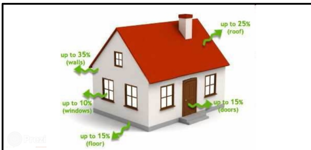
Figure 5. The lost of energy as a result of poor insulation in buildings
