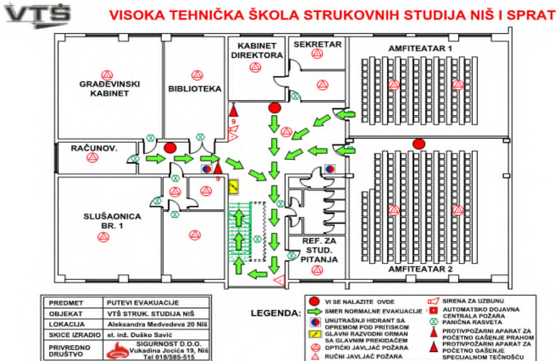
Picture 4: Evacuation Plan for the I floor of the College of Applied Technical Sciences Nis
