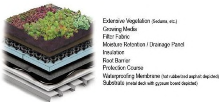
Figure 1: Layers of extensive green roof
