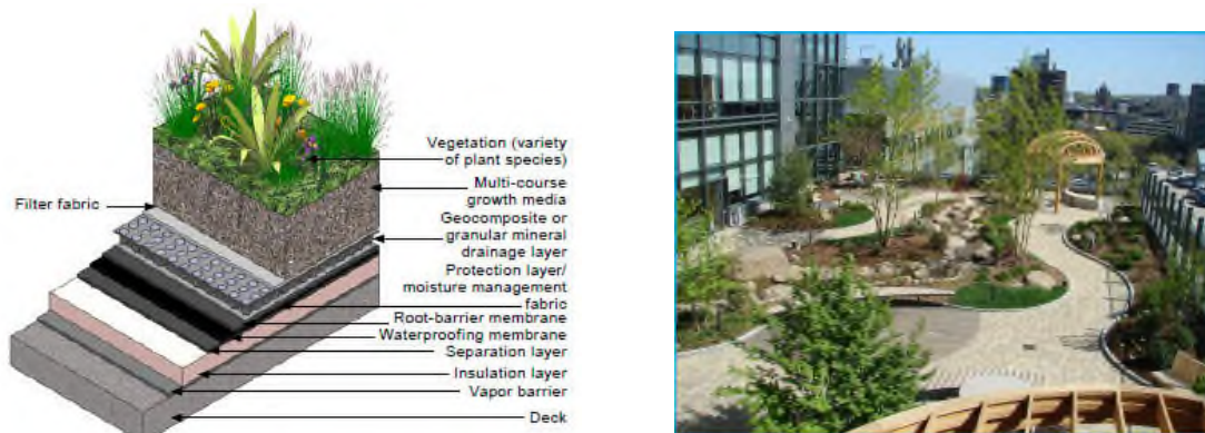
Figure 2: Layers of intensive green roof
