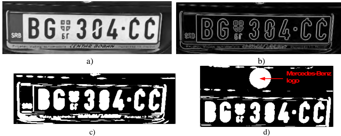
Figure 3: a) result after removing noise using Median filter b) result after detecting edges using Sobel operator c) result after applying basic morphological operations d) eliminating the Mercedes-Benz logo
