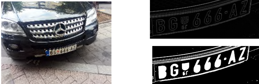
Figure 6: Detection of skewed plates and applying different morphological techniques in order to detect difference between character “G” and digit “6”
