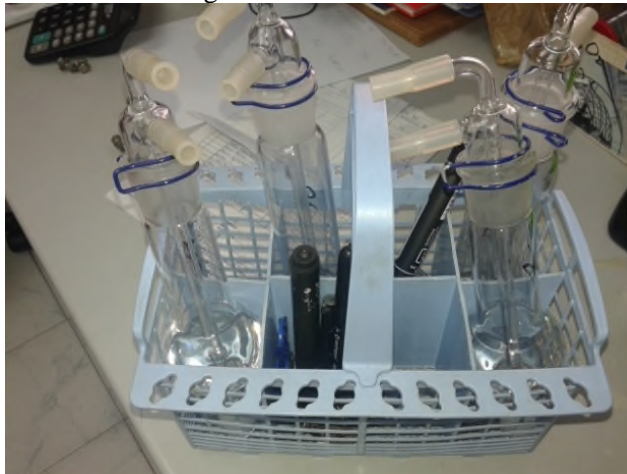
Figure 2: Gas coolers for \text{NO}_2
