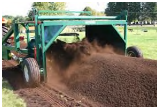
Figure 3. Machine for overturning compost piles sorted in kind
