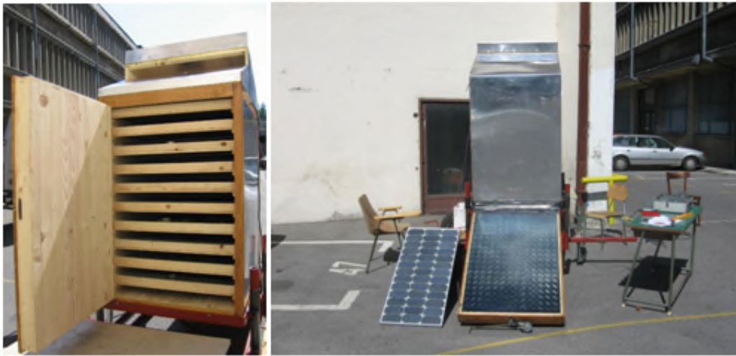
Slika.2. Modular mobile, universal, ecological, chamber solar dryers for drying biological materials [Topić]
