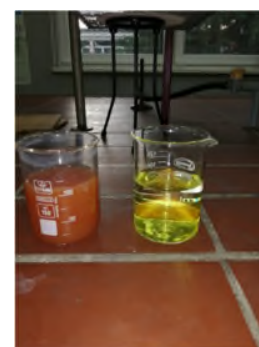
Figure 20. Endpoints titration for determining carbonate hardness
