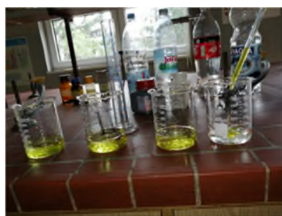
Figure 19. Titration with HCl solution
