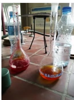
Figure 18. Endpoints titration for determining chloride
