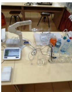
Figure 15. Probes for pH - value, electrical conductivity and ion selective electrodes
